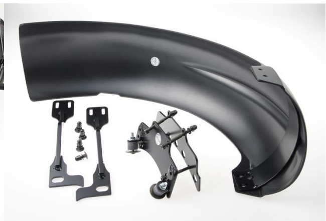
Abb. 3 – swinging rear incl. mounting material
