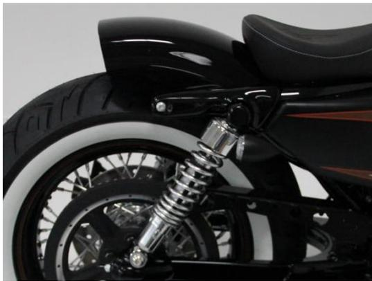
Abb. 1 – Mounted fender, fender struts and indicator set
